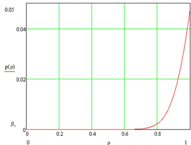
**Figure 10.** Impact of the sensors density on the losses
